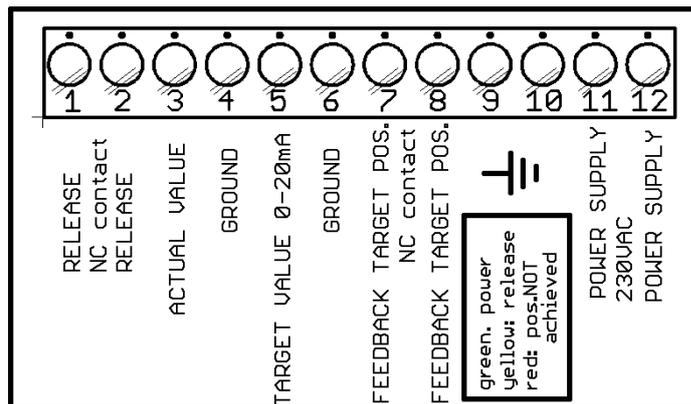
The supply voltage should be connected to terminals 11...12 as indicated in the connection diagram on the housing cover.
