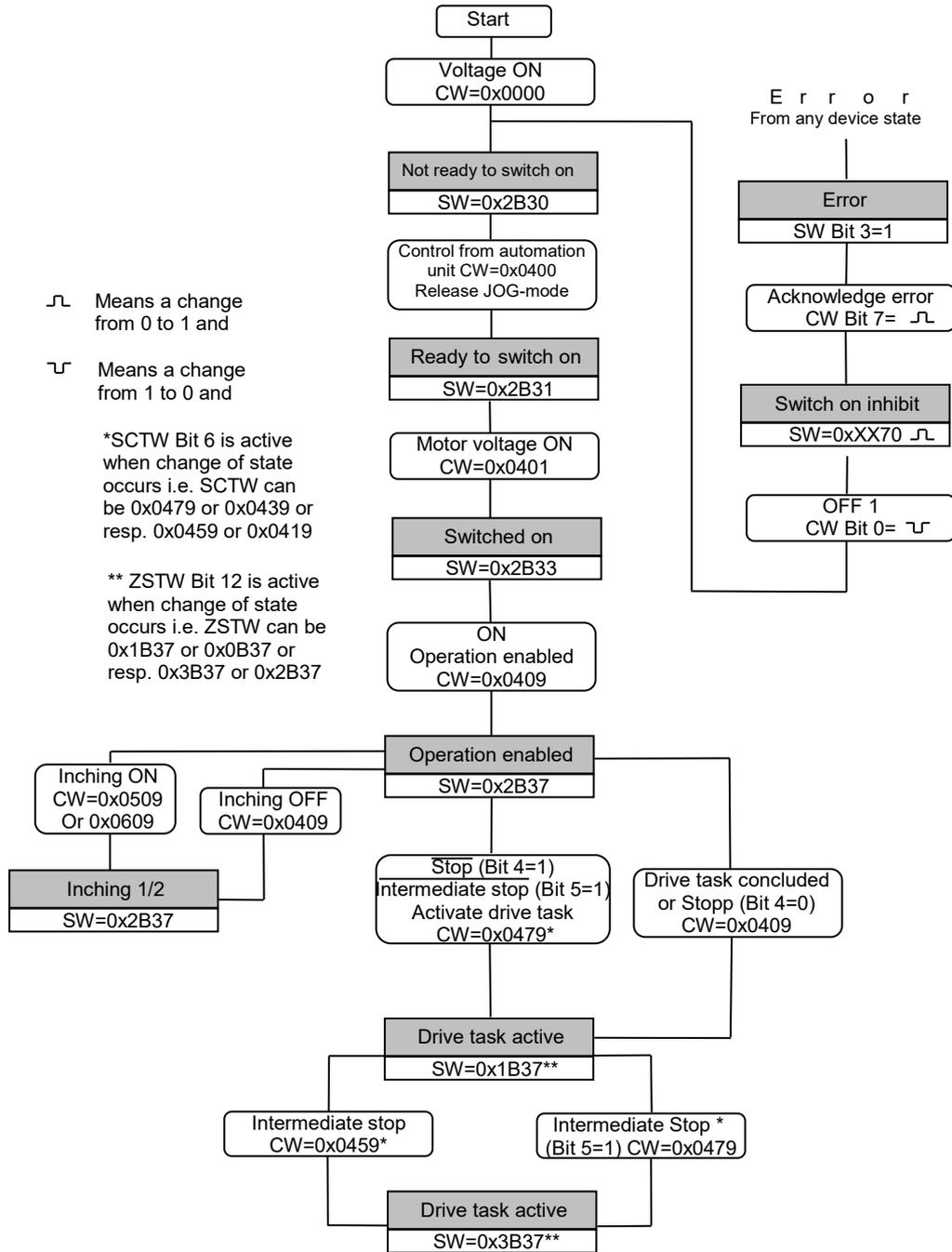
Figure 5-1: Functional diagram of control mechanism, positioning operating mode
