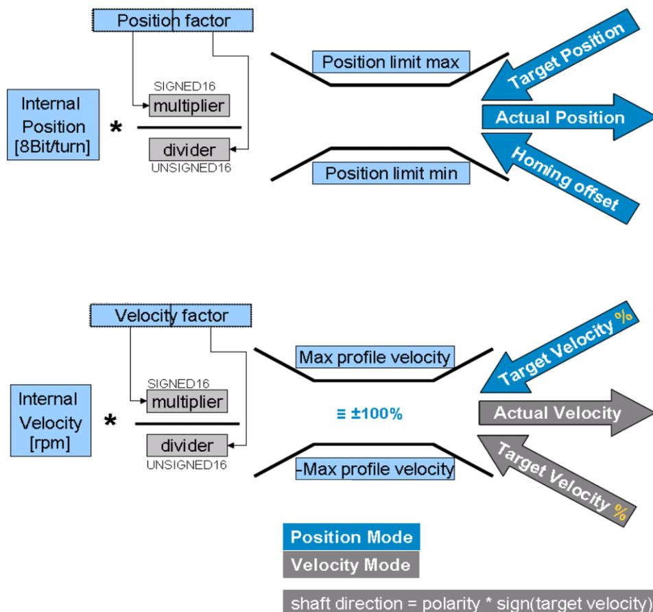
Figure 7-1: Position and velocity scaling
