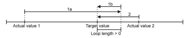
If the target value is above the current position (actual value 1) and the loop length is > 0, the drive runs past the target value by the specified loop length (run 1a) and then runs to the target value (run 1b).
