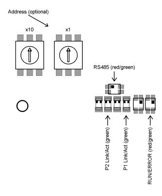
The LEDs are visible through two windows even when the bus adapter cover is closed.
