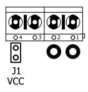
The former is generally selected if the motor power supply is run in a safety circuit with the EMERGENCY STOP and the databus has to remain active during an EMERGENCY STOP, or if the motor power supply does not permit correct operation of the bus adapter due to inadequate voltage stability or high interference voltages.
